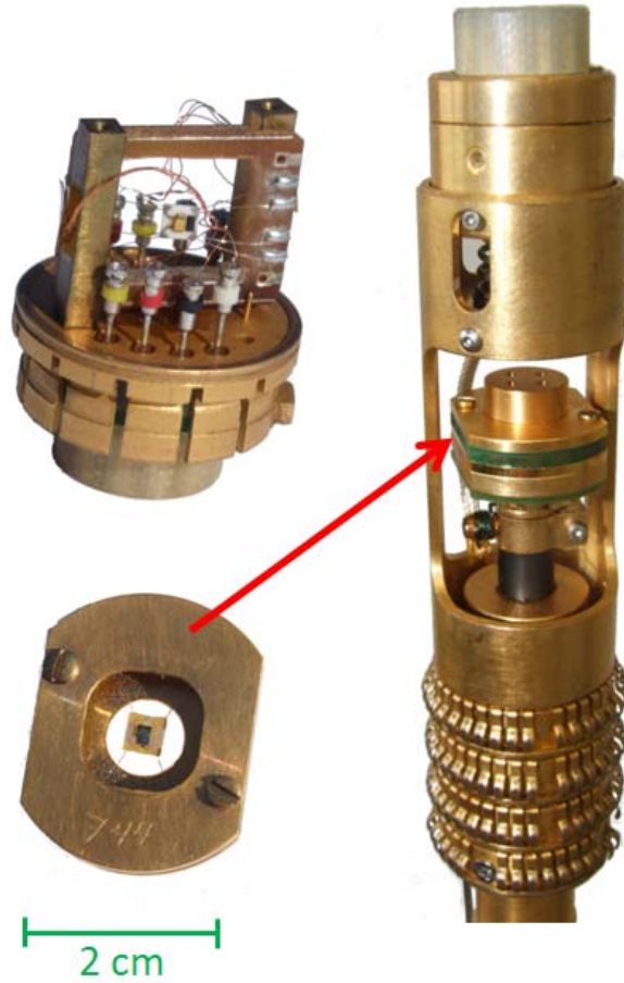
Fig. 24: The left upper part: modified commercial puck for vertical HC measurement with the heater and thermometer on the corundum plate, ^3\text{He} puck with the sample; the right part: ^3\text{He} insert with the puck for HC measurement.
