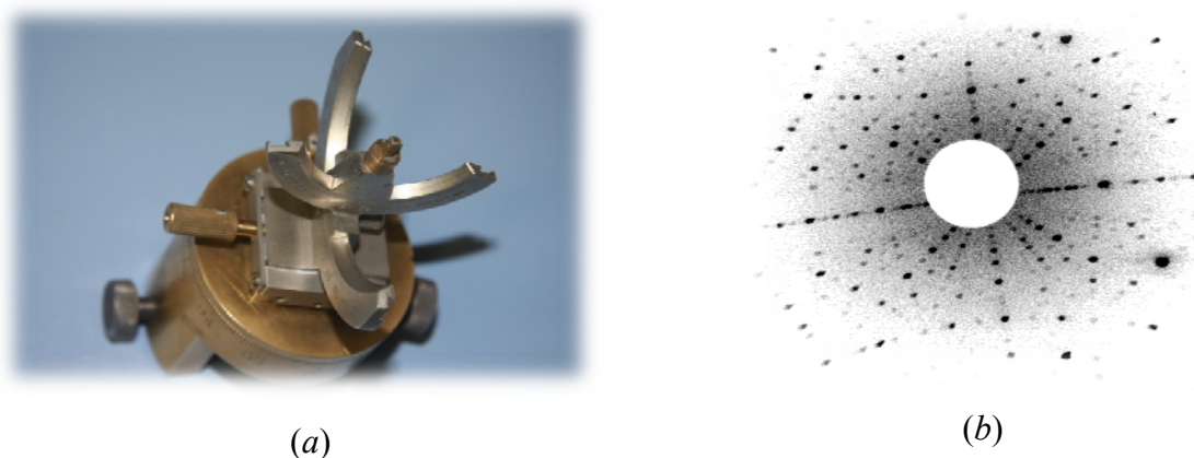
Fig. 20: Goniometric head (a) and Laue pattern (b) of CeRhIn 5 single crystal with the a -axis oriented perpendicular to the image plane.
