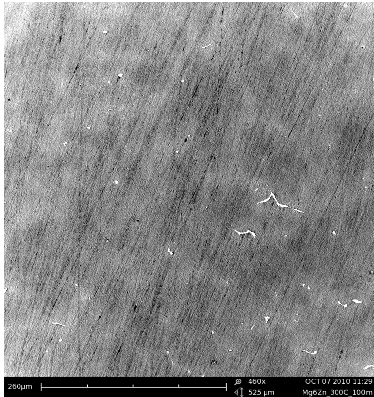
Figure 4.4: SEM image of Mg6Zn alloy annealed at 300 °C for 100 min.
