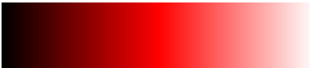
Figure 3: Red hue with maximum degree of saturation ranging from minimum to maximum brightness (from left to right).
