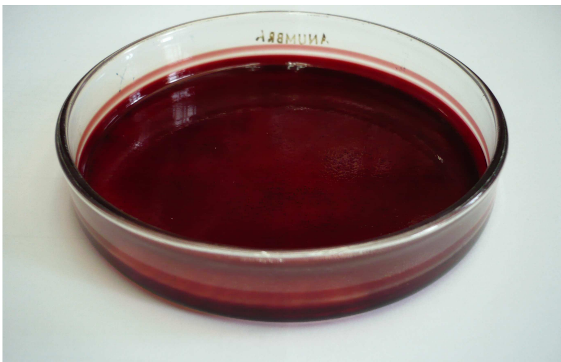
Fig. 27.: Prepared Cu(TPP) membrane in Petri dish
