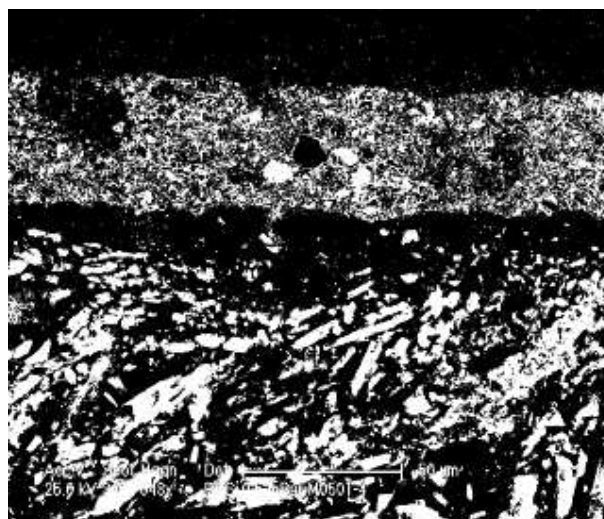
Fig. 2.9: Binary image of particles of vermilion, white lead, clays, and particles with a high contents of carbon black corresponding to the intensity range of 255-50 in the M0501-4 sample.
