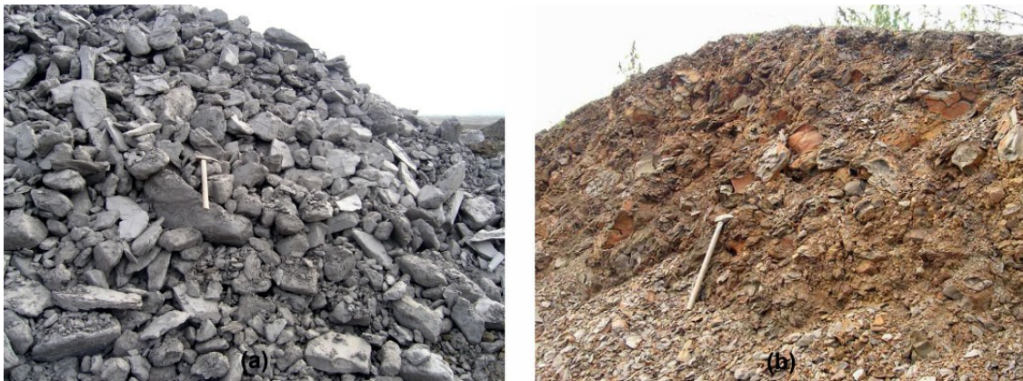
Fig. 2.3: Landfill during filling process (a) and after 10-15 years of self-weight consolidation (b).
