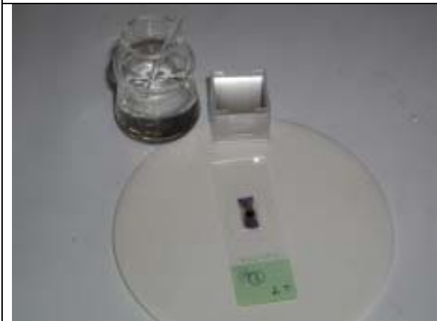
Fig 129. Stained and dried preparation is covered by Solacryl.
