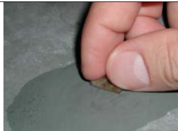
Fig 119. During grinding with sandpaper with 1200 and 2000 grain, pressure is applied very gently to avoid formation of grooves on the sample surface. After finishing grinding, the section is rinsed with water and left to dry.
