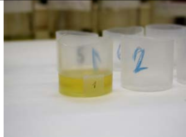
Fig 109. Embedding media in marked thin-walled flat-based containers.
