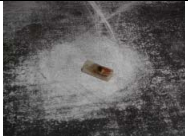
Fig 116. Grinding of bone-implant section with sandpaper from lower to higher grain size (Grain: 100, 200, 240, 800, 1200, and 2000).
