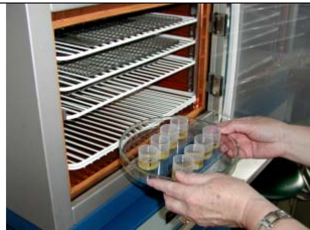
Fig 111. Curing process first at 37°C, then at 60°C for 3 to 5 days.
