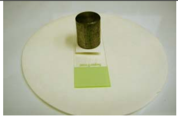
Fig 122. The glued on section has a weight load applied for about 12 hours. After hardening of Solacryl, it is possible to grind the section from the other side. (in the case of using superglue it is possible to grind immediately).
