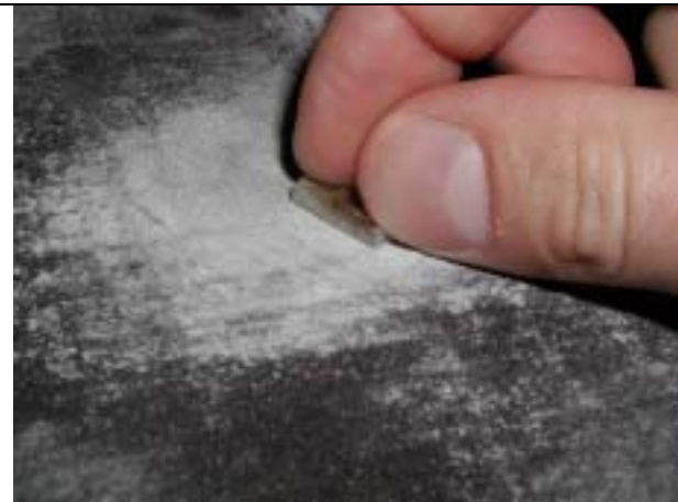
Fig 117. Manual grinding of bone-implant section.
