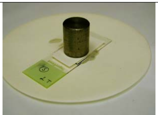
Fig 132. After mounting, a small weight load is placed on top of the cover glass for one day while the Solacryl dries and hardens, in order to keep the section flat. (This prevents distortion of the preparation).
