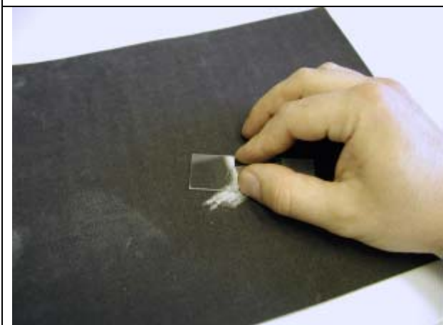
Fig 125. Grinding of the glued bone-implant section to the slide by sandpaper.
