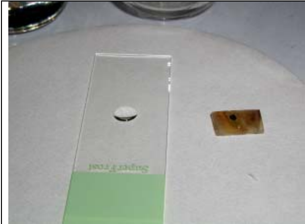
Fig 121. On the underlay surface of the slide, and on the polished surface of the prepared section Solacryl is placed (it is possible to use superglue.) This causes the polished surface of the section to stick to the underlay surface of the slide.
