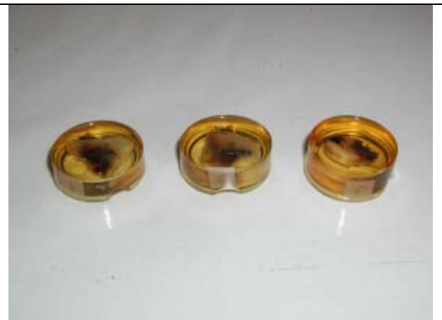
Fig 112. Cured blocks ready for cutting.
