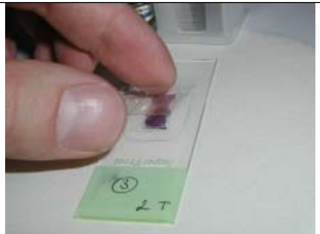
Fig 130. Application of cover glass (mount).
