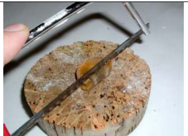
Fig 114. Sectioning a bone-implant specimen to the thickness of 1-2 mm using a metal saw.
