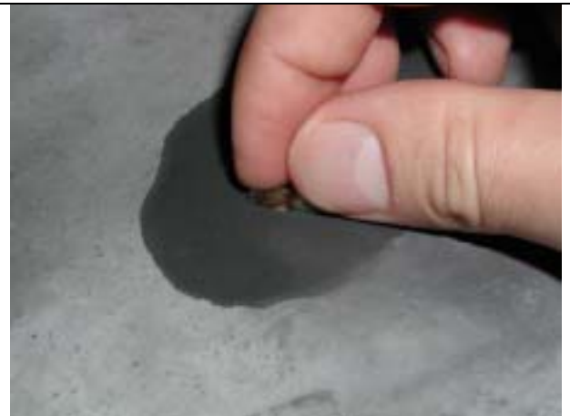
Fig 118. During grinding with sandpaper with the 1200 and 2000 grain, it is better to moisten sample with water.
