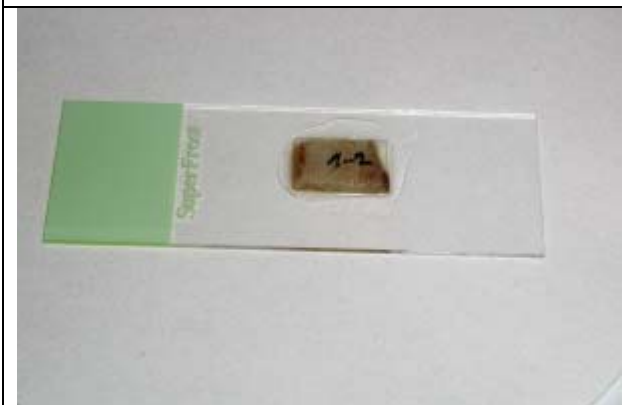
Fig 123. The glued on bone-implant section is ready for grinding.
