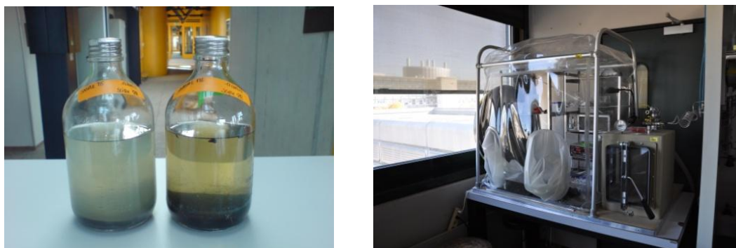
Figure 10. Sediment microcosms and handling glove box chamber.
