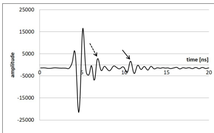
Fig. 4 Signal response from the soil with marked uppermost horizon lower boundary (dotted arrow) and E horizon lower boundary (black arrow)
