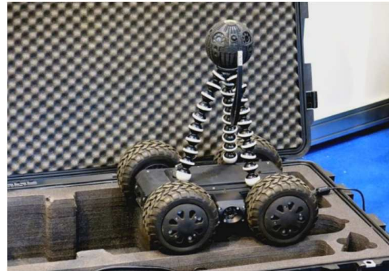
Reconnaissance and inspection complexes Scarab (bottom) and Sphere (top)
