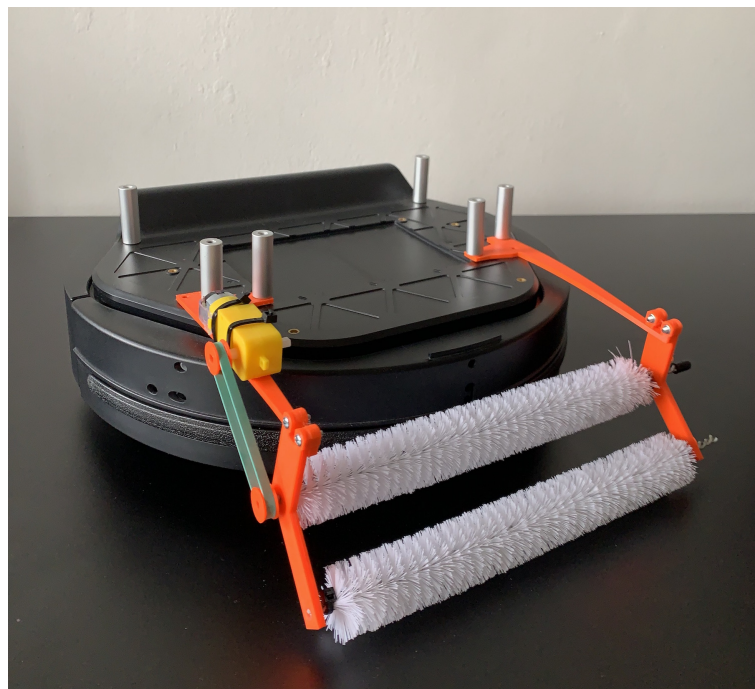
Figure 6.13: 3D printed prototype of picking mechanism.
