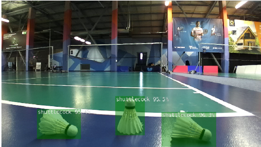
Figure 6.3: Multiple shuttlecocks detected on real badminton court
