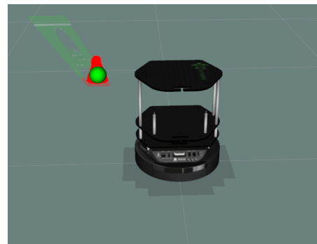
Figure 6.6: Estimated position of shuttlecock, from RViz
