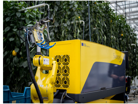
Figure 3.10: Closeup of end manipulator
