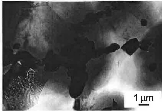
Figure 6.59: TEM micrograph of the as cast QE22 magnesium alloy showing particles of Mg_3 (Ag, Nd) phase.
