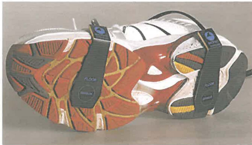
Figure 26. Pressure transducers in shoe sole. Obtained from: ( http://www.biopac.com/ProductImages/ss28.gif )
