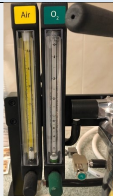
Figure 3.1 Setting of an oxygen flow of anesthesia system.
