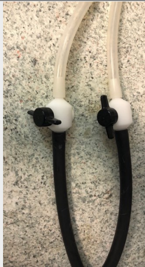
Figure 1.3 Hoses with switches connecting anesthesia system to the induction chamber and imagine station.
