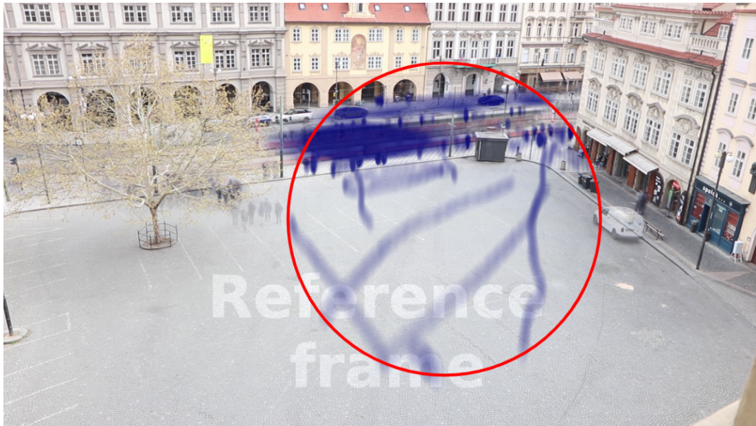
Figure 4.2: An example of a detections heatmap. The highest density of detections is at the tram stop.
