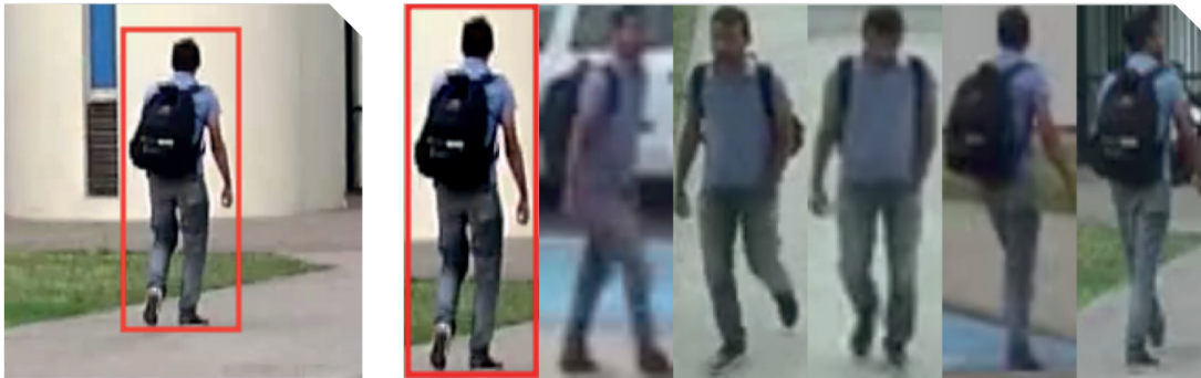
Figure 1.6: Figure showing one use case of the VICTORIA system - tracking a person that carries some object of interest. The first picture is the queried person, the second one is the results of the query - the same person in different places, tracked by multiple cameras. The original picture can be found at https://www.victoria-project.eu/fileadmin/websites/victoria/documents/180517-victoria-flyer_6-faces_Final.pdf .
