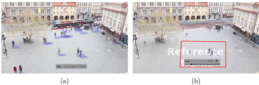
Figure 2.3: An example of a detection query. The image on the left shows a screenshot from a stream while the image on the right shows detection crops as query results.
