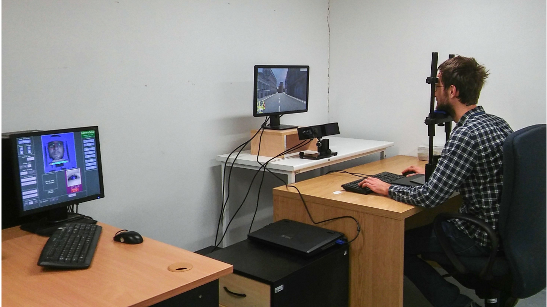
Figure 1.2: Example of a desktop VE setup with eye tracker SR 1000
