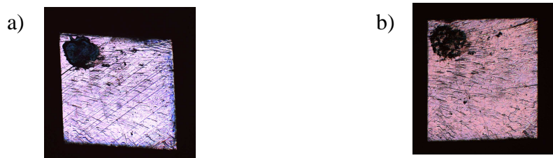
Fig. 6.5: Shape changes of martensitic samples during the reorientation of martensite induced by application of compressive deformation on green face. The shape of the sample in variant 6 (a) and macroscopic shape of the sample in variant 1 (b). Images of green face.
