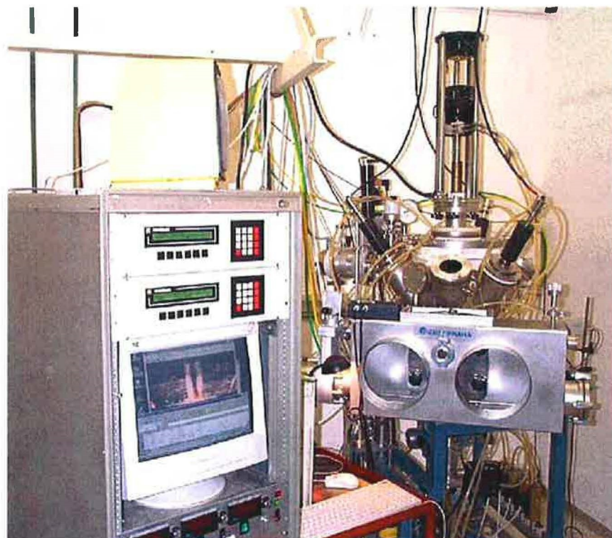
Figure 3.2: Tri-arc furnace from outside.
