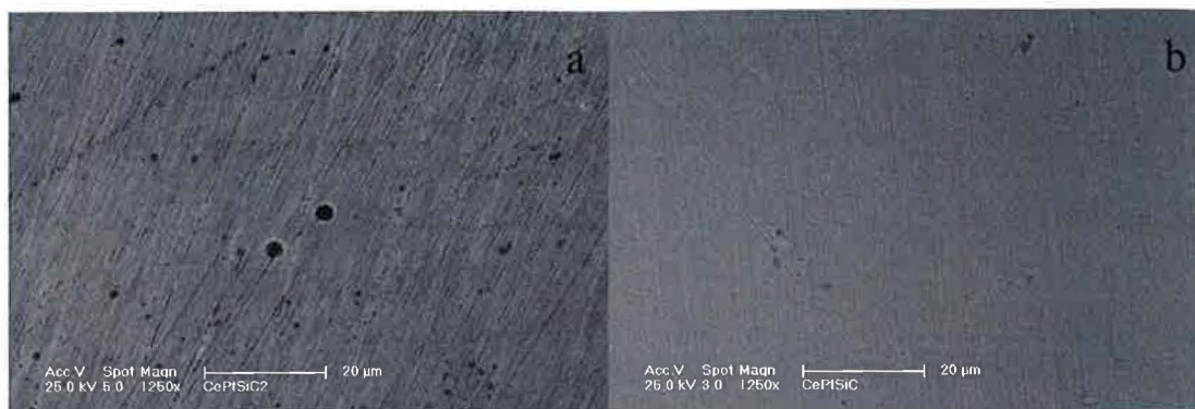
Figure 8.48: SEM micrographs of CePt_3Si_{1-x}C_x . a - x = 0.2 of C, b - x = 0.5 .
