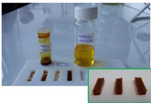
Figure 17: The copolymer BAFKU 41 –HMS 064 after preparation as bulk material (small vial), as re-melted material in the shape of platelets (see inlay; another re-melted sample is visible in the large image while still being in the mould), as solution in chloroform (large vial: dissolved piece of re-melted material).
