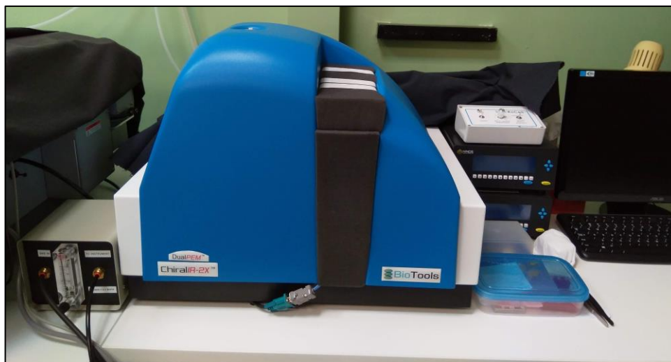
Figure 5.1: Spectrometer ChiralIR-2X TM used for the measurement of VCD and IR spectra. (VCD, vibrational circular dichroism; IR, infrared)
