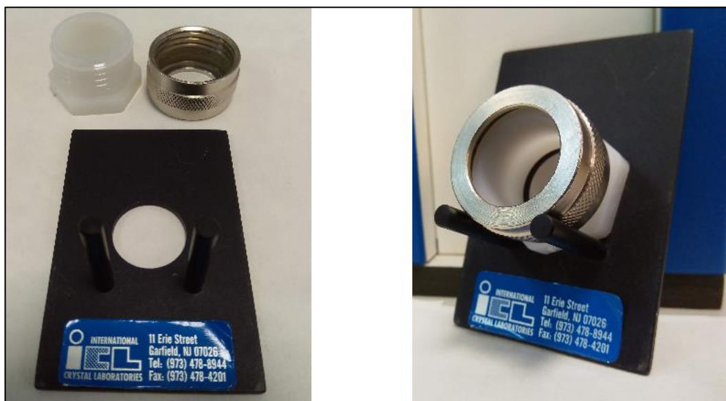
Figure 5.2: Beta Cell and a plastic cell holder from International Crystal Laboratories used for measurement on ChiralIR-2X
