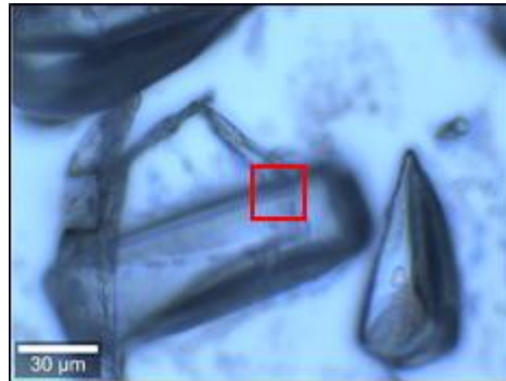
Figure 5.3: In WITec software Control FOUR, the user can select the desirable part of the image for scanning, that is marked by the red rectangle
