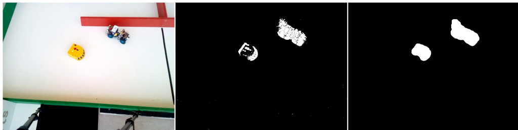
Figure 4.2: Effect of morphological operations and convex hulls on detected objects. Original figure (left), frame difference of two consecutive frames (middle), morphological opening and closing applied on the frame difference (right).
