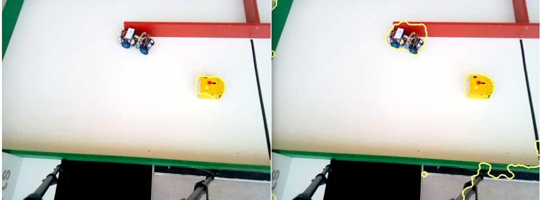
Figure 5.4: Comparison of frame differencing (left) and background subtraction (right). While frame differencing detects only the moving car, background subtraction detects also the non-moving car and other frame regions that differ from the reference image.
