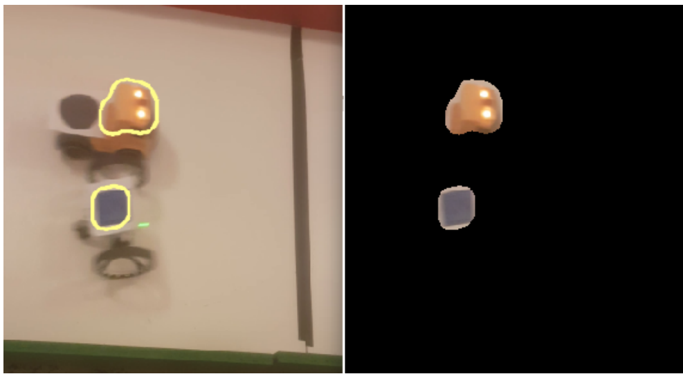
Figure 4.7: Detection of two colors with the color filtering technique – color contours (left), union of color filter masks (right).
