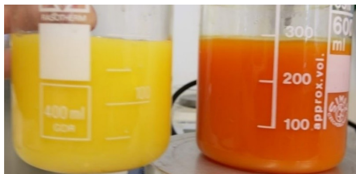
Figure 5.3 Left - Clouded PTA; right – clouded PTA after addition of Al(NO_3)_3 and citric acid
