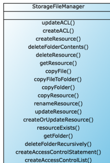
Figure 5.4: A class diagram generated directly from a TypeScript file, demonstrating an implemented FileManager abstraction
