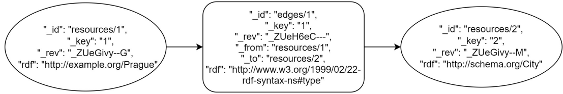
Figure 3.2: Samuelsen’s direct with edges representation of RDF for the sample data in Figure 3.1a
