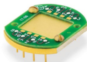
Fig. 3.6: Special puck for measurement of electric resistivity by Quantum Design [53].
