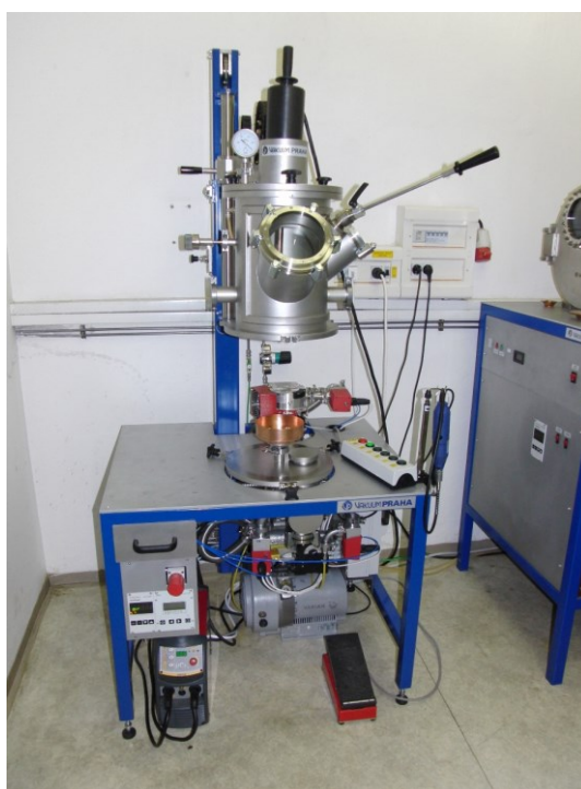
Fig. 3.1: The mono-arc furnace for preparation of polycrystalline samples [45].
