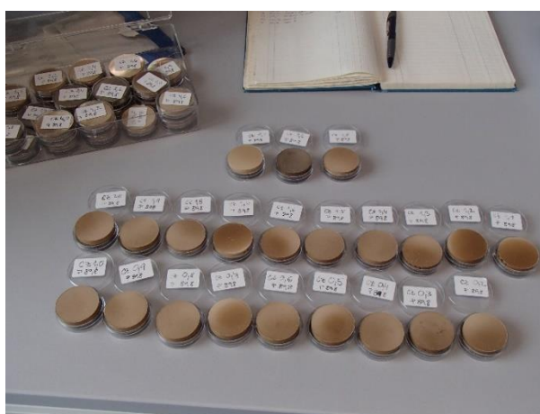
Figure 3.13: Pressed pellets for XRF of trace elements. (Photo: K. Flašarová)
