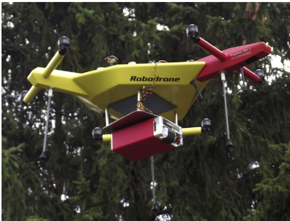
Fig. 4. Mini-airborne gamma-ray spectrometric device in flight. The set consists of a hexacopter (type Kingfisher by Robodrone Industries) and a gamma-ray spectrometer (type D230A by Georadis).
