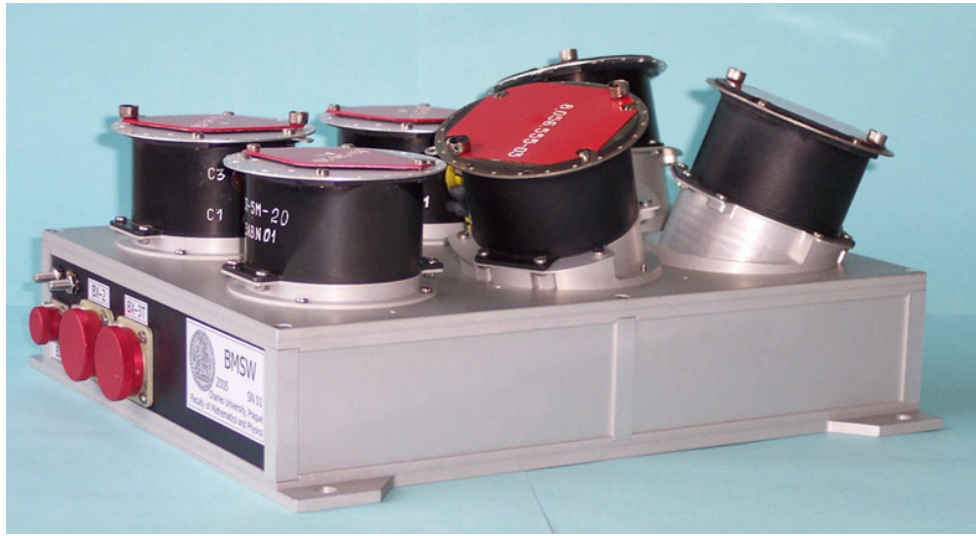
Figure 5.1: A photograph of an engineering model of the BMSW instrument. Adopted from Šafránková et al. (2013a).
