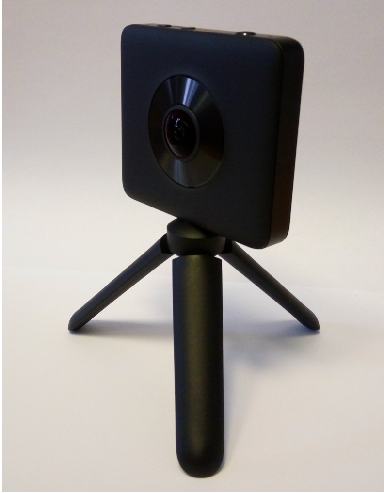
Figure 3.3: Our Mi Sphere camera. The same lens is duplicated on the other side of the camera. The camera is only about 10 \times 10 \times 2 centimeters in size, making it very portable.
