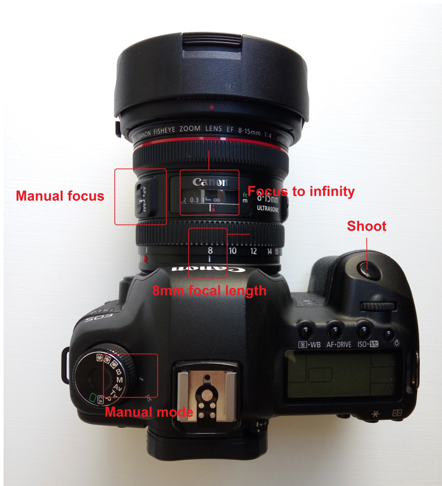
Figure A.3: Description of the camera controls on the top of the camera and the controls of the lens.
