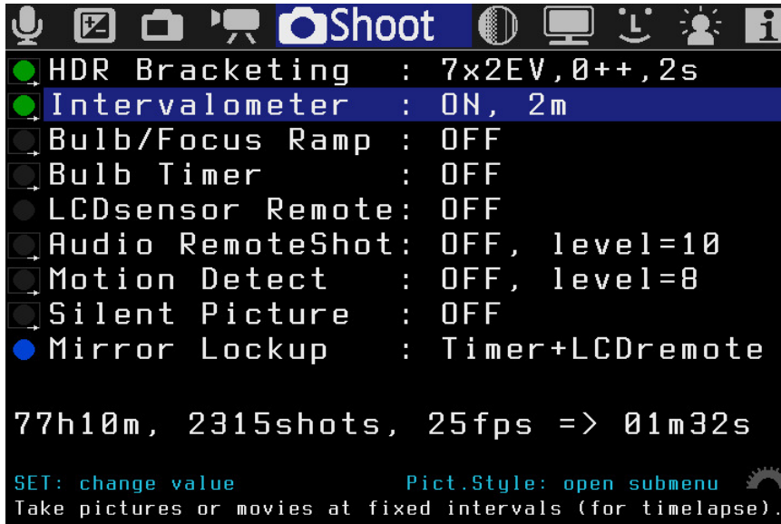
Figure A.5: Exposure bracketing and intervalometer settings of Magic Lantern software. The HDR bracketing setting signifies shooting 7 images with a 2 EV step in between each pair, starting from the darkest one and increasing the exposure. The intervalometer is set to shoot a sequence of pictures every two minutes.
