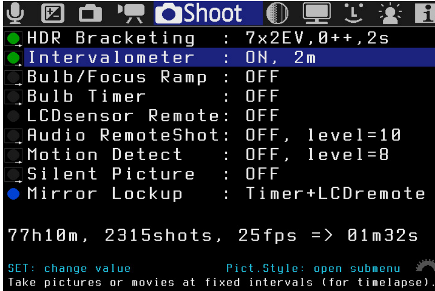
Figure 3.5: Exposure bracketing and intervalometer settings of Magic Lantern software. The HDR bracketing setting signifies shooting 7 images with a 2 EV step in between each pair, starting from the darkest one and increasing the exposure. The intervalometer is set to shoot a sequence of pictures every two minutes.
