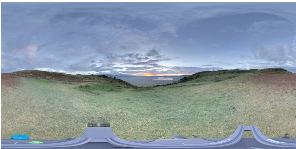
Figure 1: An example of a low dynamic range environment map. Since the map covers all 180 polar degrees, we can see the camera tripod in the bottom of the image.
