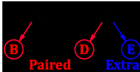
Figure 21: Example of pairing nodes during merging. Here we are merging A and C, and we are pairing their children. B and D get paired, as they are the first children of their parents. E is left as extra since there is no child of A left to be paired.
