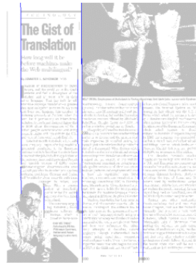
(b) Connected components grouped into vertical lines. Upon close inspection, we can see that each page column contains multiple connected components.
