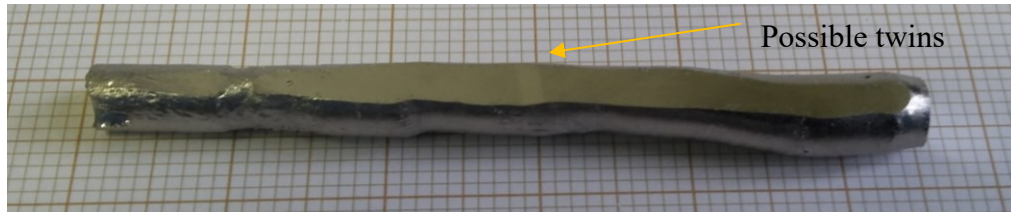
Figure 14 - Annealed rod R29.5 with polished side, showing signs of possible twins at surface.
