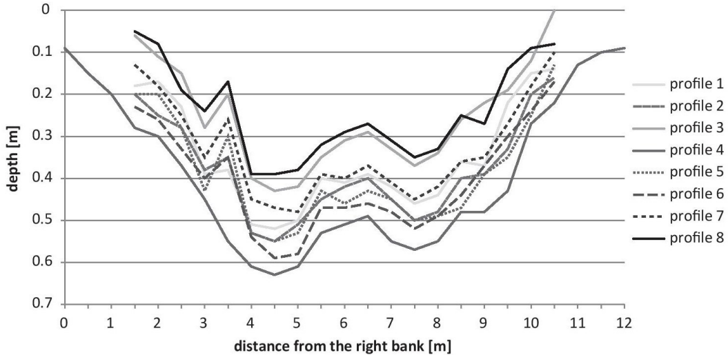
Fig. 4 – Cross section profiles of lake outflow at different water stages. Measurement time: profile 1 – 3.8. 15:30–16:00; profile 2 – 3.8. 17:45–18:05; profile 3 – 4.8. 8:00–8:15; profile 4 – 4.8. 17:20–17:40; profile 5 – 4.8. 20:10–20:35; profile 6 – 5.8. 10:10–10:30; profile 7 – 5.8. 13:50–14:10; profile 8 – 5.8. 15:00–15:15.
