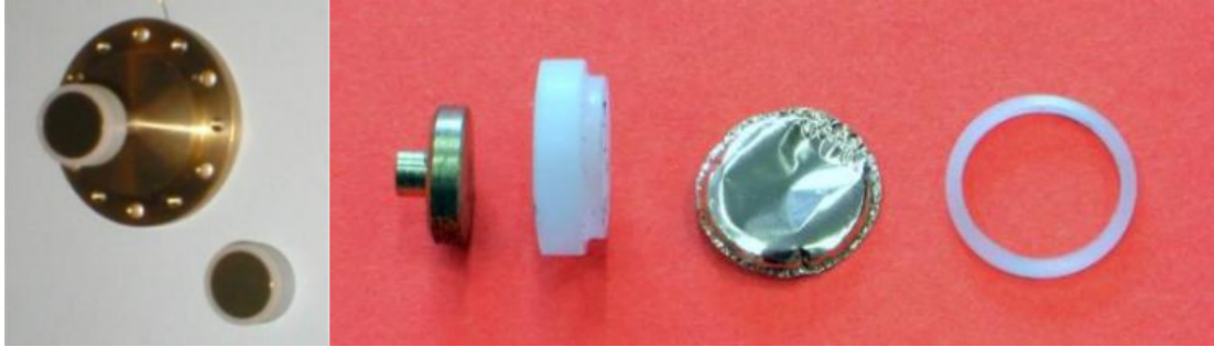
Figure 2.3: Photograph of a fully built second sound sensor (left) prepared for installation into the experimental channel. A decomposed sensor (right) made from a brass electrode, tefflon holder and gold-coated nucleopore membrane (from left to right, respectively).
