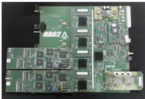
Figure 5.2: A TEL62 board equipped with two TDC boards and the quad gigabit board [60].
