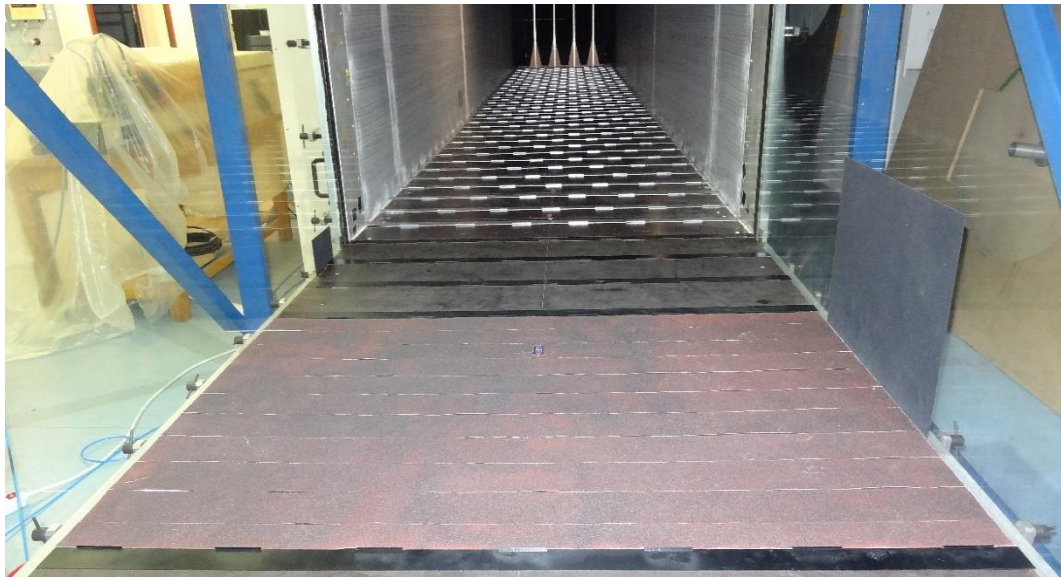
Figure 1. Simulation of a rural area in the wind tunnel.
