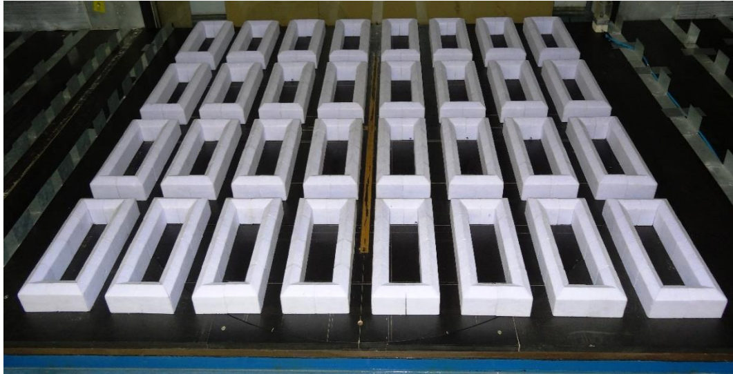
Figure 13. Idealized urban area placed in the wind tunnel.
