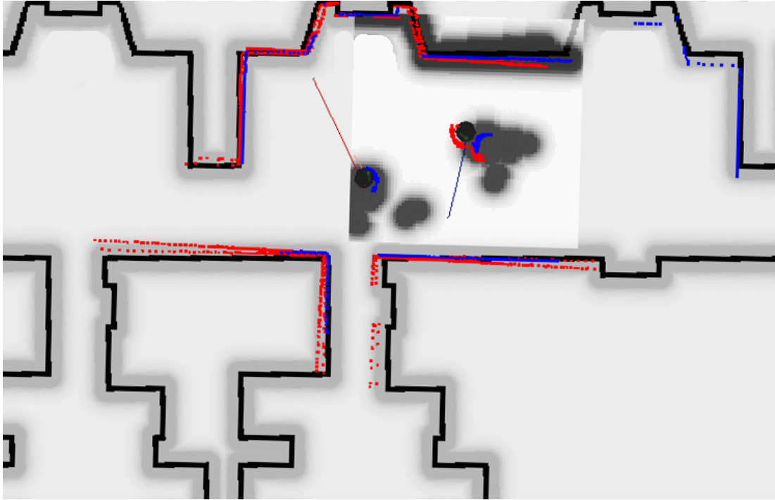
Figure 12.3: A Robots' perception of the environment. Back rounds are the robots. Red and blue dot clouds are the laser scanner reflections. Red and blue path is the path planner output. Shades of gray, forming also the black wall line, represent local and global costmap.
