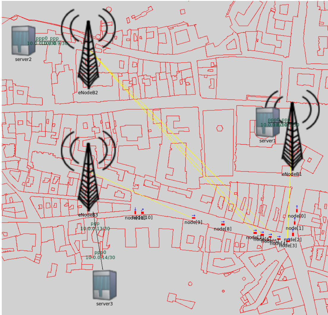
Figure 2.4: An example of a graphical output of the Veins simulation. Cars cooperate using LTE connection in the streets of the Lesser Town of Prague. Red rectangles with blue arrow represent cars and their direction of movement. Yellow beams represent ongoing wireless transmission.
