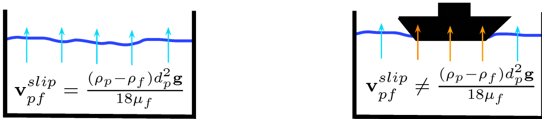
Figure 2.3: Correct behaviour on the left side and non-physical behaviour on right - penetrating of the ascending particle through the boundary having different orientation that the particle-flow.
