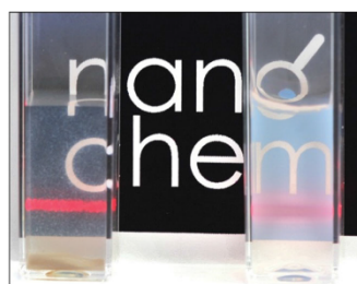
Figure 4. Photography of ND1 and ND4 dispersions ( 0.5 \text{ mg mL}^{-1} ) in PBS, 30 min after mixing. ND1 (left) precipitates and finally gives sediment at the bottom of the tube, while ND4 (right) remains in the form of stable colloid scattering the laser beam (red laser pointer).
