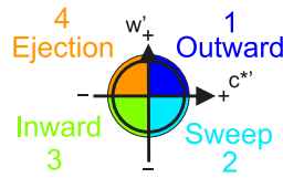
Figure 1.13: The scheme of event definitions used in turbulent flux quadrant analysis.
