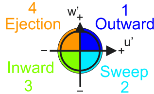
Figure 1.11: The scheme of event definitions used in velocity fluctuation quadrant analysis.
