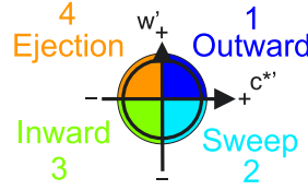
Figure 4.7: The scheme of event definitions used in quadrant analysis of turbulent pollution flux.
