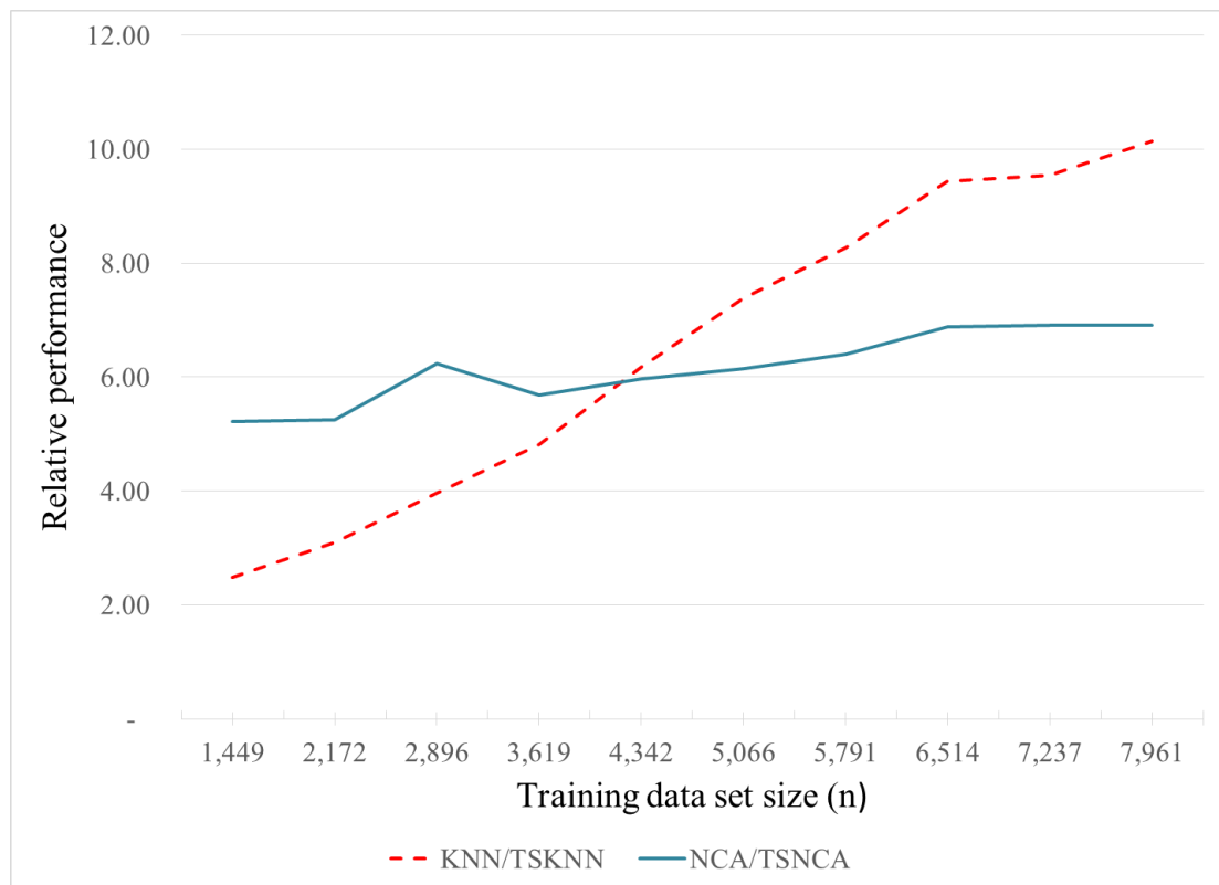
Figure 5.1: Relative performance ratio of computer time in training sessions for KNN and TSKNN, and for NCA and TSNCA, respectively.
