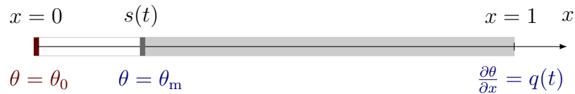
Figure 2.2: Formulation of the one-dimensional Stefan problem for a discretized solution. Heat flux through the left end of the bar q(t) is given by the analytical solution.
