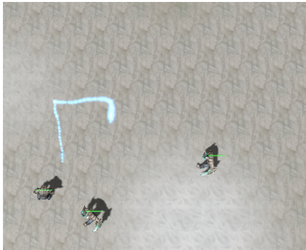
Figure 3.6: The blue glowing line in the image represents the drawing. While the player holds the mouse button, the mouse positions are repeatedly sampled and projected to the surface. The projection points are then added to the line and the space between the points is filled with a blue glow dots to show the line.
