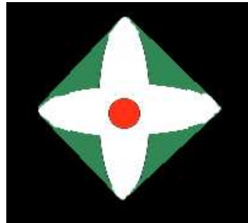
Figure 3.7: Illustration of the definition of the term hollow. Both green and red areas are not parts of the object but the red area is completely enclosed by the object and thus it is not considered to be a hollow.
