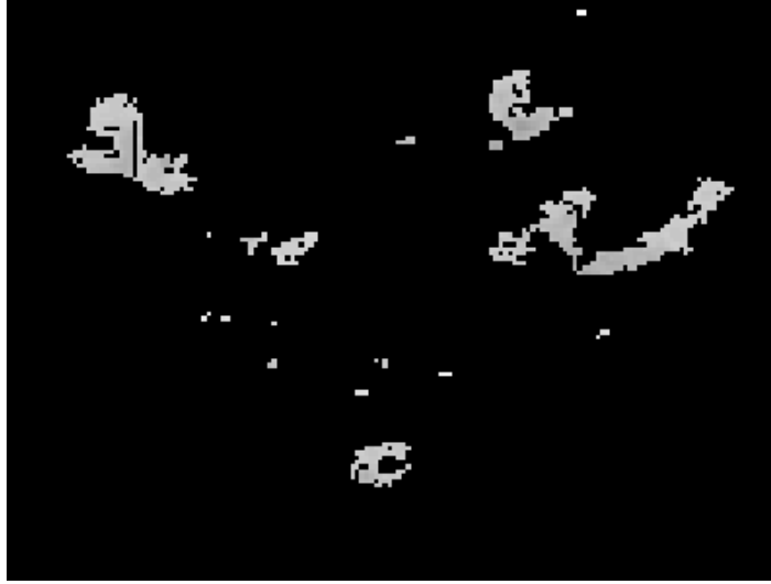
Figure 3.5: The figure demonstrates the result of thresholding based on median value when applied on the output image of the basic thresholding.
