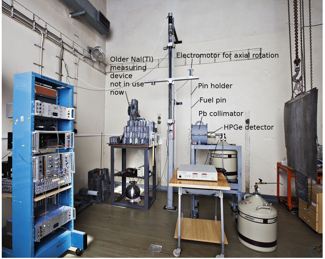
Figure 3.6: The laboratory with gamma spectrometry systems for fuel pins measurement. [7]
