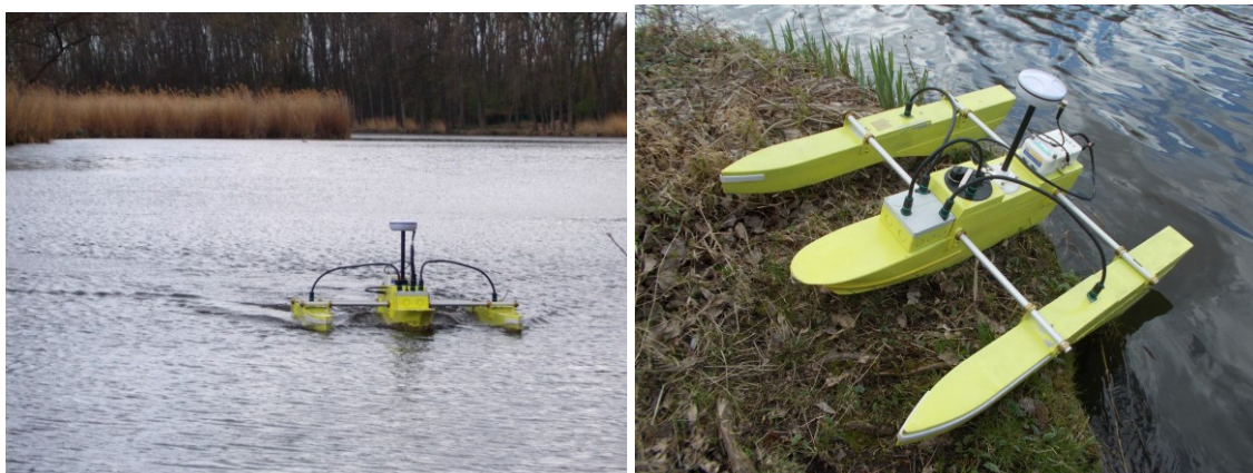
Figure 16: Bathymetric measurement with RiverSurveyor (photo L. Beranová)
