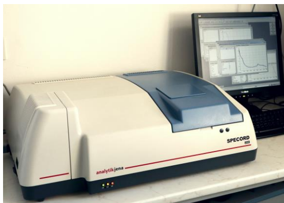
Figure 3.17. Photograph of the spectrophotometer (Specord 250) used for measurements of absorption spectra.
