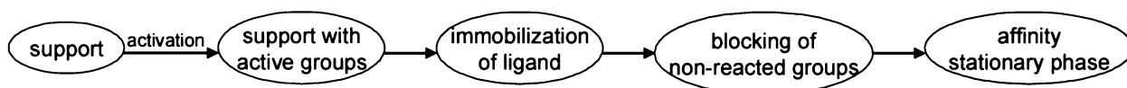
Fig. 2.4: A scheme of a procedure for preparation of an affinity stationary phase.
