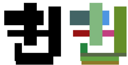
Fig. 24. The convolution kernel used in the experiment (left) and its FER decomposition into 10 blocks (right).
