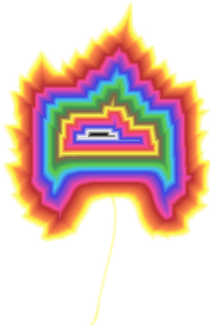
Fig. 5. The distance transform of the leaf image. The pixels are labeled by pseudocolors according to the DT values.
