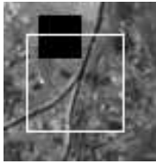
Fig. 7. Explanation of the boundary effect. The inside pixels near the template boundary (white square) are affected by the pixels from the outside of the template if the scene is blurred. The extent of this effect depends on the blur size (black square).
