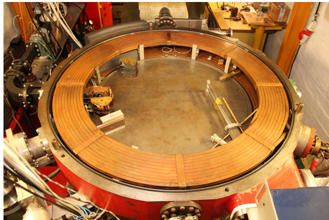
Figure 4.2: View inside the vacuum chamber
