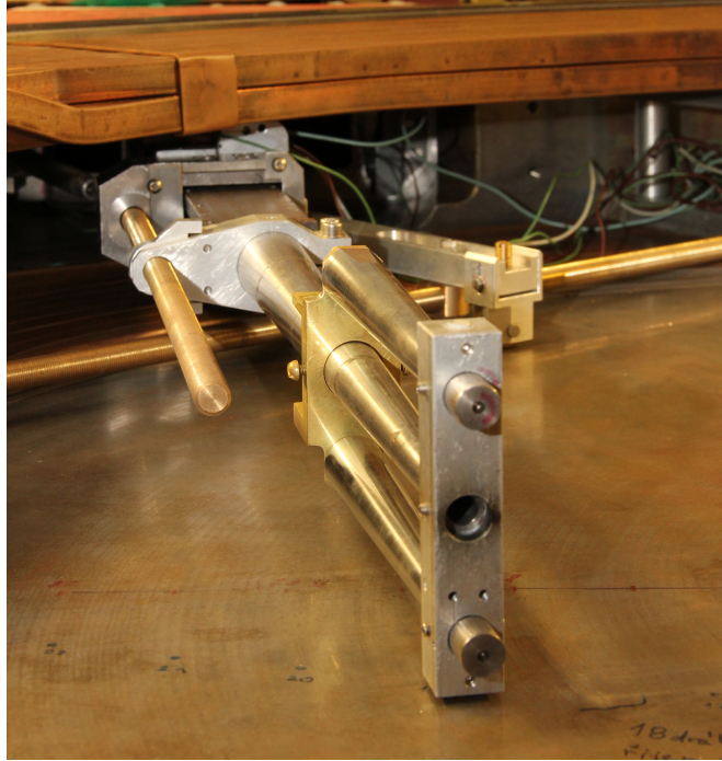
Figure 4.4: Adjustable iron channel for electron extraction
